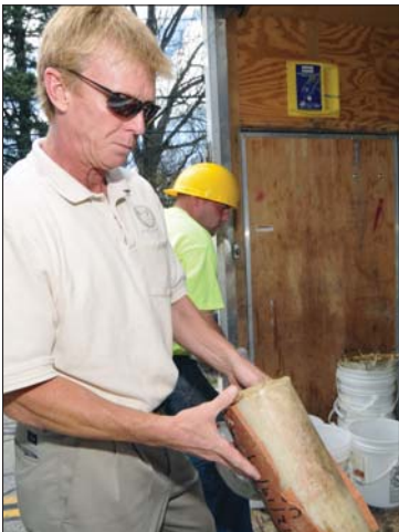
City engineer Bob Kelly examines a sample of CIPP lining. The city collects neighborhood data for about a year to develop the most cost-effective I&I solutions available.
